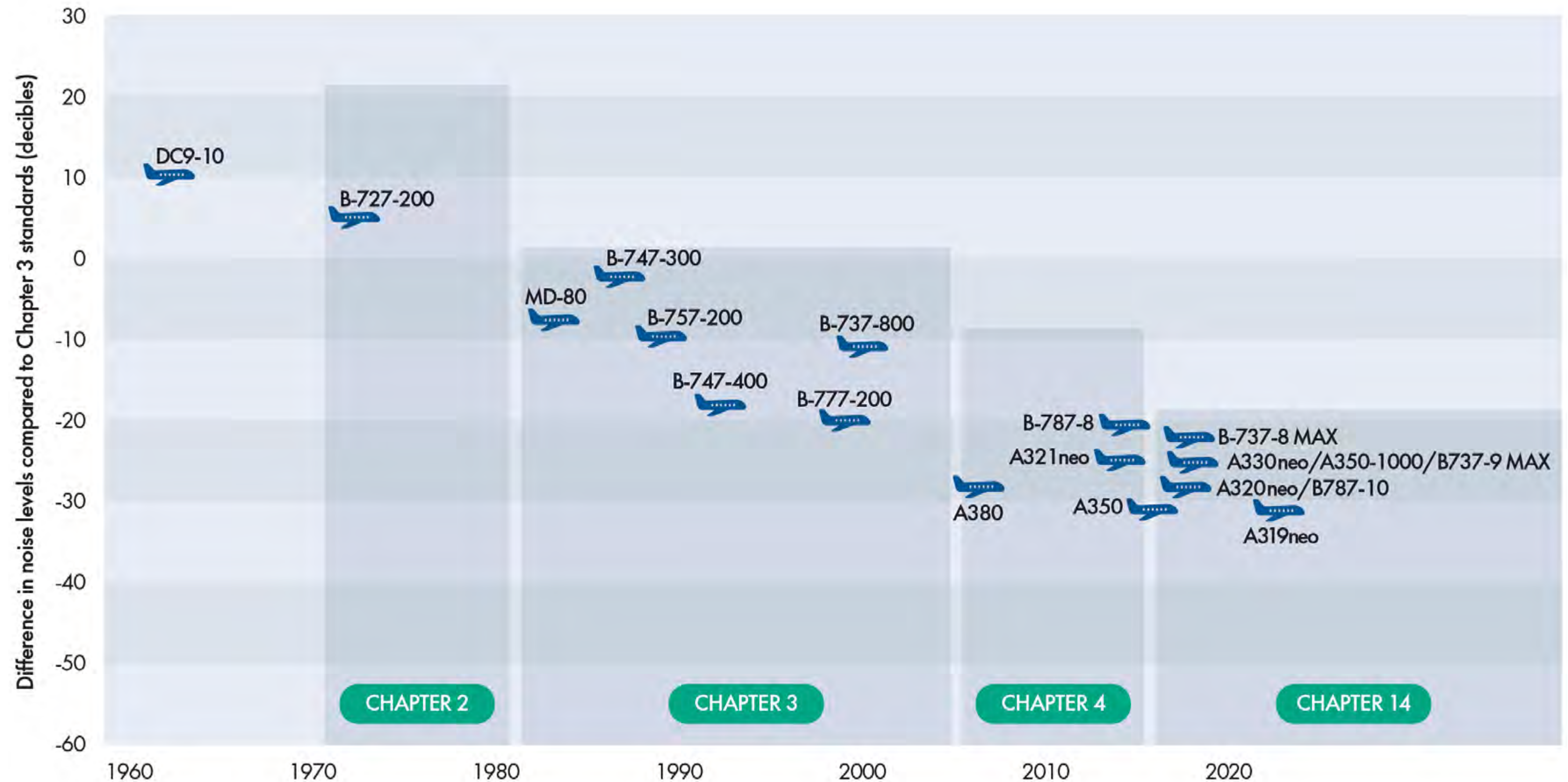
Figure 8. Downward trend in the noise certification of aircraft (Source: ICAO noise database 4 )
