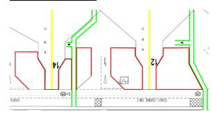
The current head-of-stand GSE parking areas (boxes bordered in a single white line) have been replaced with boxes bordered in a single white line with a new inner red line.
